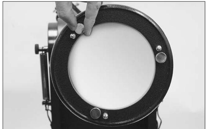
**Figure 17.** The tilt of the primary mirror is adjusted by turning one or more of the three larger thumbscrews.
