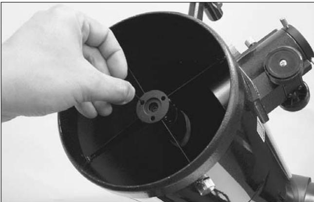
**Figure 15.** Adjust the tilt of the secondary mirror by loosening or tightening the three alignment set screws with a 2mm hex key.
