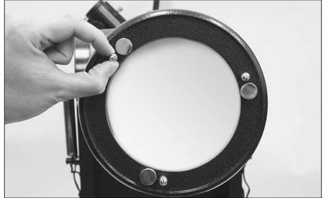
**Figure 16.** The three small thumbscrews that lock the primary mirror in place must first be loosened before any adjustments can be made.
