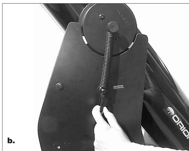
**Figure 8. (a)** To attach the spring to the base, grip the pull loop with your index finger and pull down on the spring. **(b)** While pulling down, slip the end ring of the spring over the bolt head and onto the narrow part of the nylon spacer, then release the pull loop.
