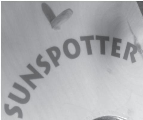
*In aiming, the Sunspotter is adjusted so that the shadow of the gnomon disappears.*
