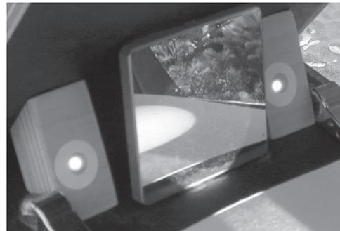
*After adjusting to make the gnomon's shadow disappear, carefully adjust the position of the Sunspotter in its cradle to center the dots of sunlight in the targets.*
