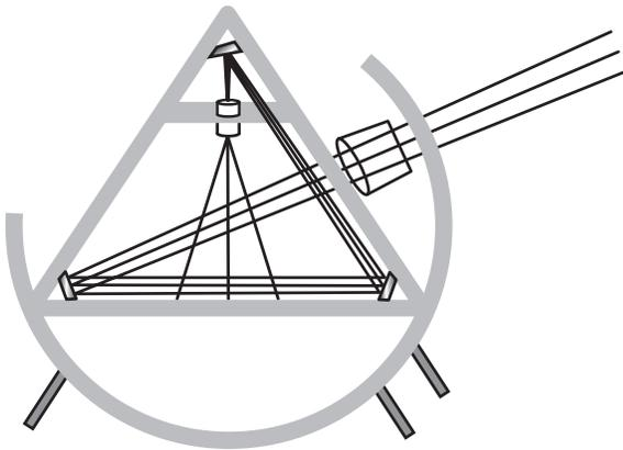
The triangular telescope enclosure has an aperture to admit the sun's light. Centered in the aperture is the telescope's objective lens. The sun's rays pass through the objective lens into the enclosure. The lens is large and achromatic, resulting in a bright, clear image. This lens is made of two separate lenses of
